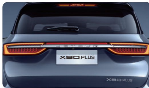
Taillights filled with 236 LED particles
